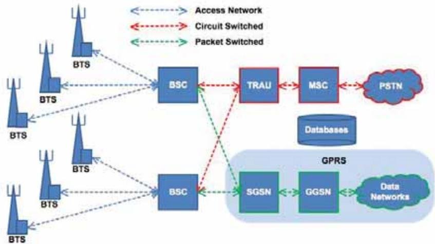
Figure 1: Network architecture of a 2G (GSM) and 2.5G (GPRS) mobile network
