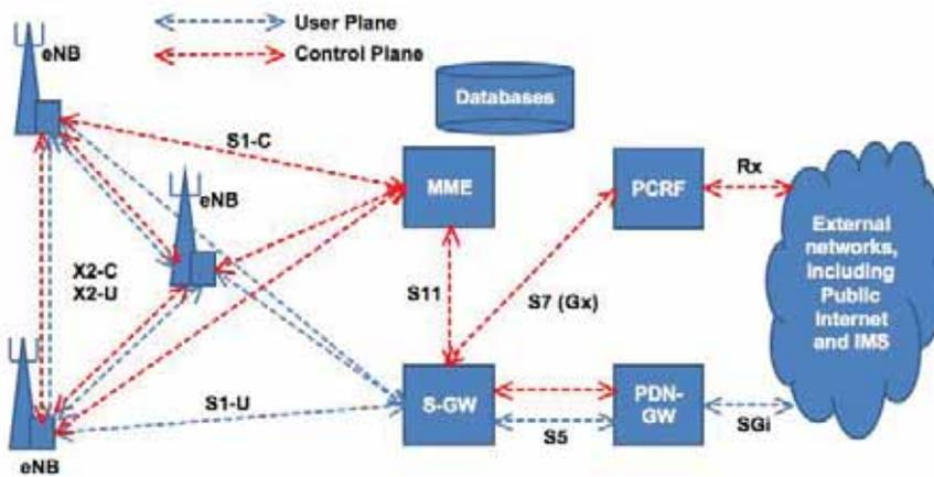
Figure 6: 3GPP Release 8 4G (LTE) network architecture
