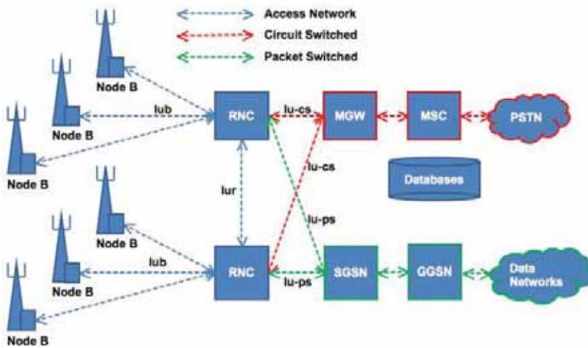
Figure 2: 3GPP Release 99 3G (UMTS) network architecture
